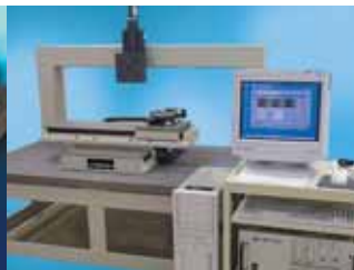
Printhead Inspection Station
