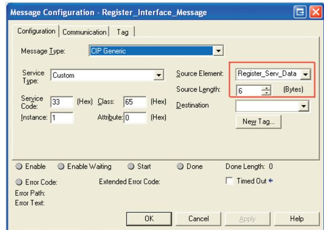
The value 100 is the register to write to, and the value to be written is 7. When the MSG block is activated, the register query is sent to the Soloist via the EtherNet/IP protocol.
