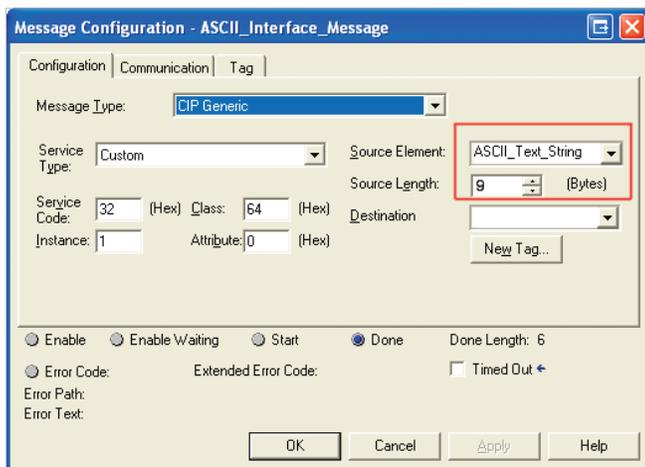
ASCII\_Text\_String (specified in the red box in Figure 2) is an RSLogix “tag”. The value of this tag is the ASCII command that will be sent to the Soloist. The example in Figure 3 shows the command “HOME X Y” as it would be configured in RSLogix.
