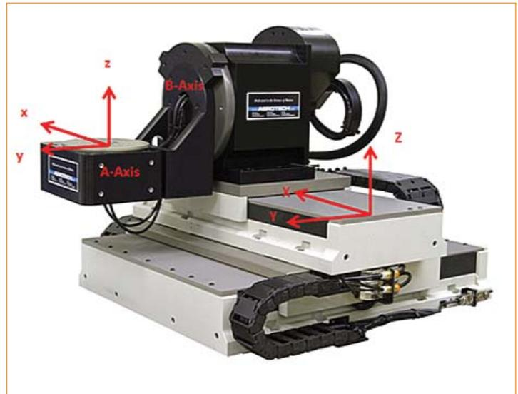
Figure 4. An example of a five-axis system showing axis orientations.
